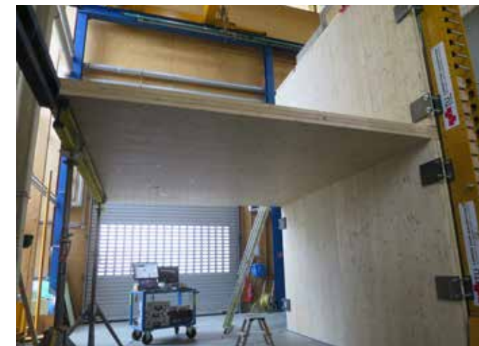
JOINT INSULATION THICKNESS K_{ij} [dB] MEASUREMENT AT THE TU IN GRAZ
